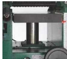
**Central Column** The thickening table is supported by a sturdy central column for superior stability and easy rise and fall adjustment.
